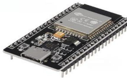
Figure -3 ESP32 development board used as the ECG acquisition and serial transmission node.
