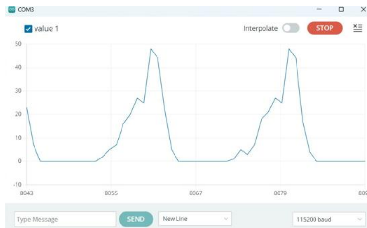
Figure -4 Real-time ECG waveform captured from the AD8232 sensor via the ESP32 microcontroller.
