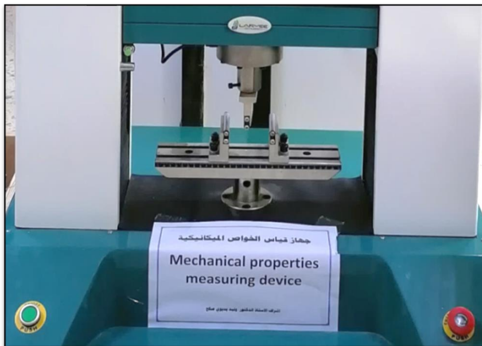
Figure -4 Bending testing device
