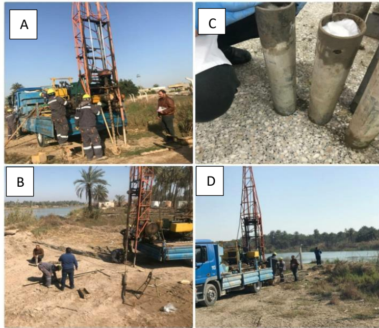
Figure -3 Images for study area represent field investigations stage where A- represent sampling of disturbed samples (DS), B- standard penetration test (S.P.T), and C&D are represented undisturbed samples (US)
