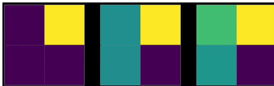
From the left to the right: picture input, output from the QASM backend, and output from the IBM Lagos backend. The real quantum computers gives the same answer as the computer simulation. (2 Data Qubits).
